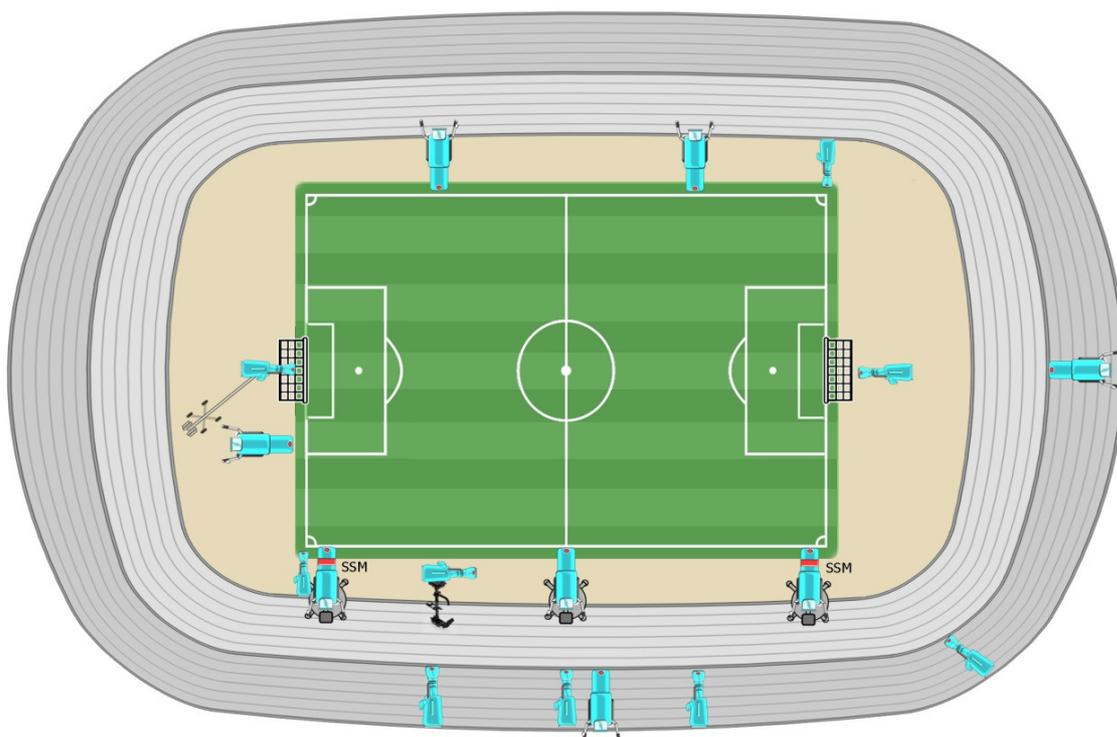
**STANDARD C:** CONFIGURAZIONE 10 TELECAMERE HD + 2 TELECAMERE IN/OUT
